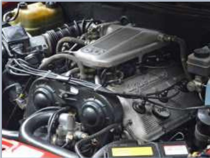
The V6 engine, so desirable when new, later brought extra headaches, especially if it had been through a sequence of owners who hadn't kept up with its maintenance schedule. The main problem was due to head gasket failure which caused oil leaks.<sup>2</sup>
